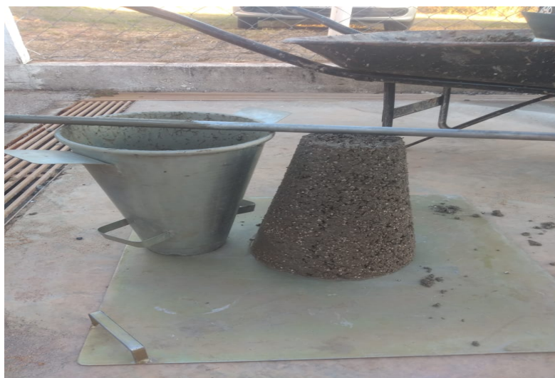
Figura 10: Slump Test - Concreto 100% EPS
